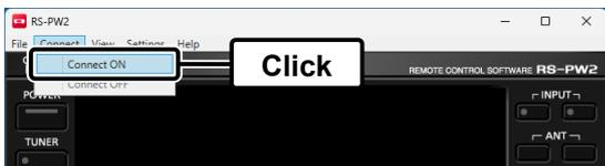
This is the first screen displayed when the RS-PW2 with connection settings (pp. 2-1, 3-1) is connected to the IC-PW2. You can remotely control the IC-PW2 by placing the mouse cursor on each key or display on the operating screen and clicking.
