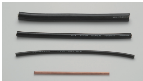
Figure 03-1. Various thicknesses of coaxial cable (From the top, 8D-FB, 5D-2V, RG-58A/U, and RG-402/U (Semi-rigid))
