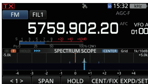
Figure 02-5. Automatically adjusts the frequency to correct any deviation with AFC
