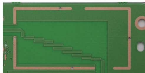
Figure 06-4. BPF installed in the next stage of mixer circuit
