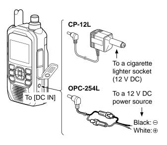
**CAUTION: BE SURE** to attach the battery pack before connecting the DC cable.
