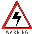
Your Icom radio generates RF electromagnetic energy during transmit mode. This radio is designed for and classified as “Occupational Use Only,” meaning it must be used only during the course of employment by individuals aware of the hazards, and the ways to minimize such hazards. This radio is NOT intended for use by the “General Population” in an uncontrolled environment.
