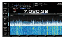
Spectrum scope with waterfall (wide screen setting)
