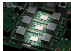
6kHz, 3kHz and 15kHz 1st IF filters (from top to bottom)
