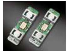
ZF-Filter (6 kHz, 3 kHz)
