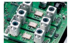
Hi-spec 1st IF filters (Roofing filters)
